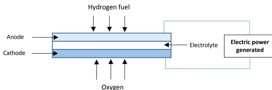
The electrodes are usually made of small platinum particles (which act as a catalyst to promote the reaction) supported on porous carbon. However, due to a number of disadvantages including the high cost of platinum, other electrode materials are now being developed.
