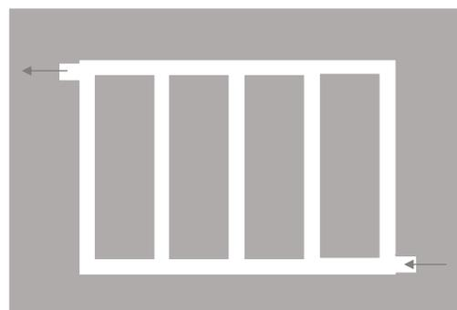
surface of the electrodes. These channels are designed to offer a large surface area for adequate gas flow while at the same time maintaining a sufficient contact surface area between the bipolar plate and the electrodes to which it is connected.
