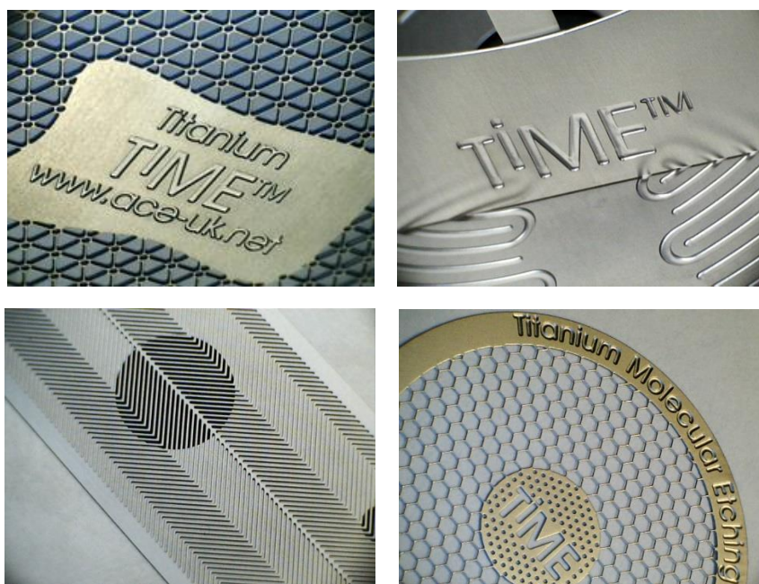
Figure 2: Titanium parts etched using the TiME process
