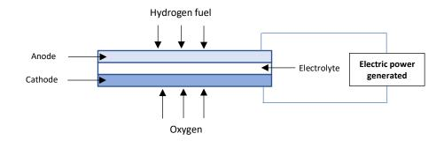
The electrodes are usually made of small platinum particles (which act as a catalyst to promote the reaction) supported on porous carbon. However, due to a number of disadvantages including the high cost of platinum, other electrode materials are now being developed.
