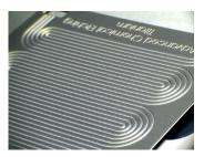
Photochemical etching can also be used to create micro-channels for miniaturized fuel cells. There is currently a great deal of interest in developing miniaturized fuel cell technology driven by advances in microfabrication technologies and also by the need to improve the performance of energy storage technologies for portable electronic devices. Photochemical etching of metal plates offers a cost-effective way of producing macro- or micro-channels for fuel cells.
